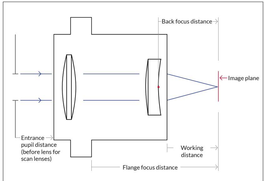
**Back focus distance** – The distance from the rear vertex of the last element to the image plane.
